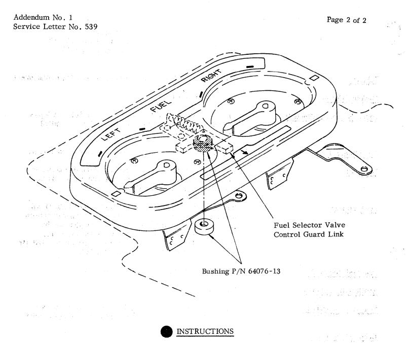
Remove fuel selector valve control handles and fuel selector valve protector plate. Remove the fuel selector valve control guard link and the bushing which is located underneath the link. Reinstall the guard link using the new bushing P/N 64076-13. Reinstall the fuel selector valve protector plate and check for sufficient clearance between the guard link and protector plate. If necessary, rework protector plate to remove any interference. Reinstall the fuel selector valve handles.
