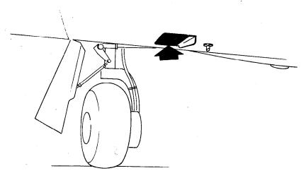
RECESSED ANTI-ICING FUEL CELL VENT
