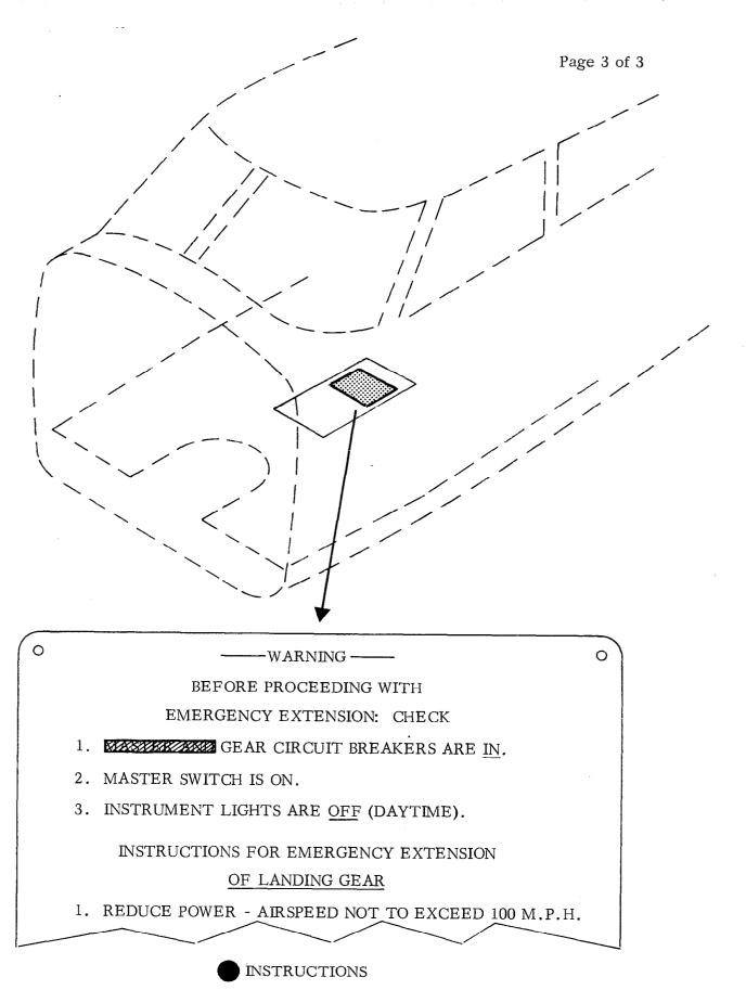
Remove the emergency gear extension access door and obliterate the words "MASTER AND" from the placard on the underside of the door with red paint.
