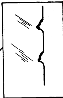
Exaggerated view of nicks in leading edge.
