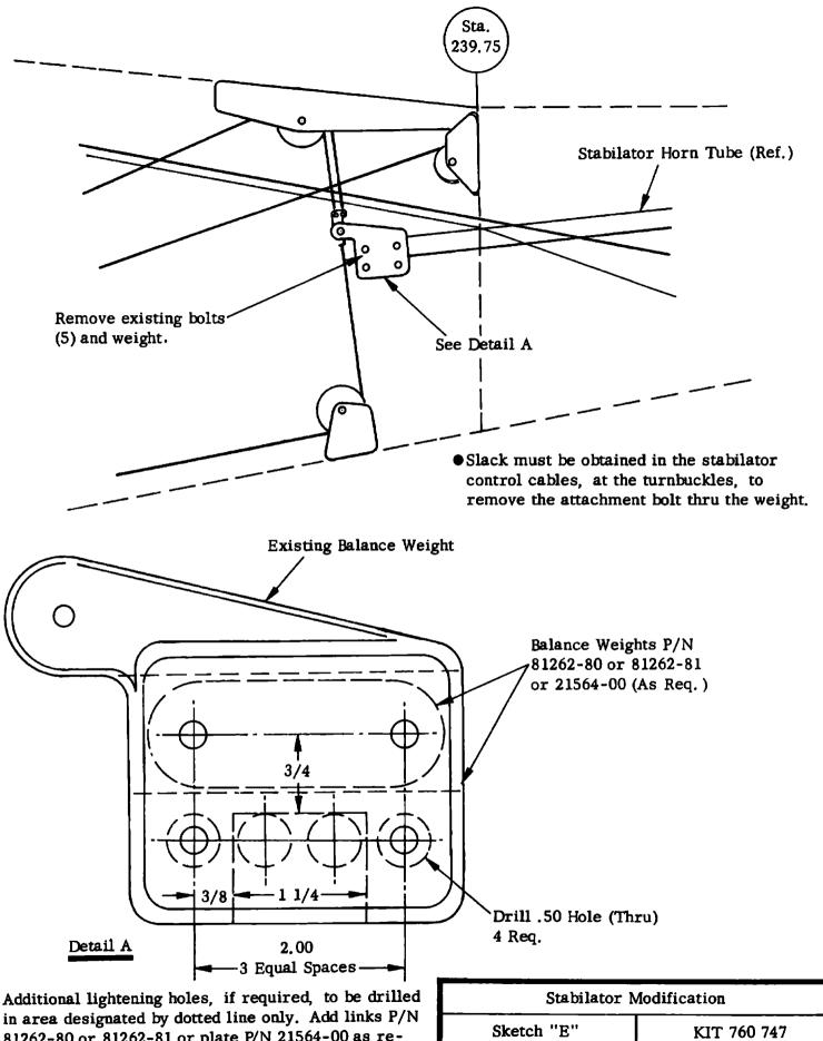
81262-80 or 81262-81 or plate P/N 21564-00 as required. Use longer bolts (AN-4) as required. The maximum weight of weight and hardware (excepting cable attaching hardware) is 3 lbs. 15 ozs. and a minimum of 3 lbs. 8 ozs.
