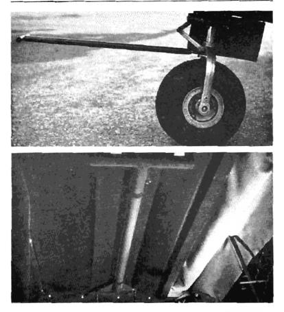
Tie-down ropes for mooring the airplane can be fastened to the wing tie-down rings and the tail skid.
