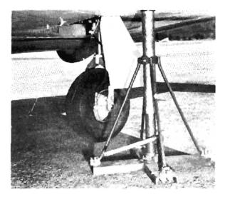
fully. Next remove the air valve core and fill the unit through this opening. Then compress the oleo to within  $\frac{1}{4}$ " of full compression, allowing air and excess oil to escape. Then reinsert the valve core and pump up the strut.
