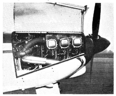
The Comanche Model 180 is equipped with a Lycoming 0-360-A series engine rated at 180 HP at 2700 RPM. The engine in the 250 is a Lycoming 0-540-A series, developing 250 HP at 2575 RPM. Both engines have compression ratios of 8.5 to 1, and require 91/96 octane minimum fuel. They are furnished with a geared starter, 50 ampere 12-volt generator, voltage regulator, shielding, fuel pump, propeller governer, vacuum pump drive, and carburetor air box and filter.
