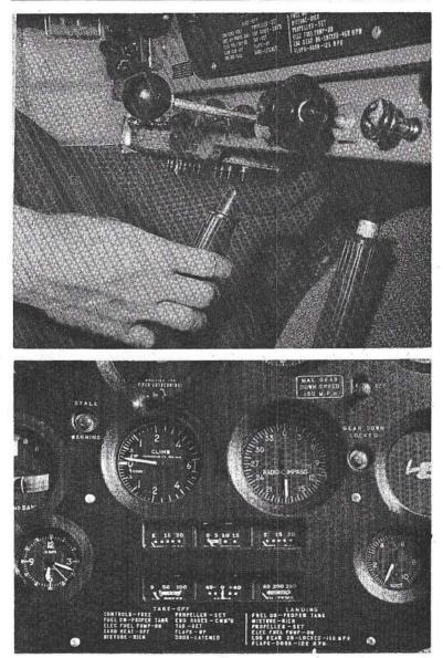
gear is accomplished with the Emergency Gear Lever aft of the nose gear well.
